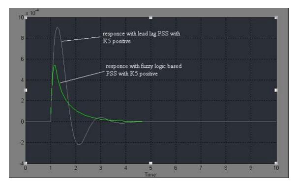
Figure 9. Comparison of angular speed with conventional PSS (lead-lag) and fuzzy logic based PSS with K5 positive
