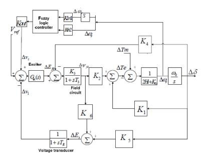
Figure 3. Implementation of fuzzy logic controller
