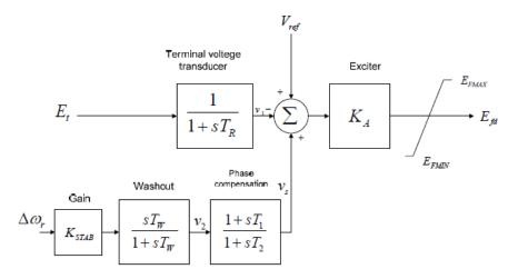
Figure 2. Thyristor excitation system with AVR and PSS
