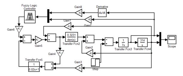
Figure 5. Simulink model with fuzzy logic based PSS
