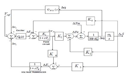
Figure 1. Block diagram representation with AVR and PSS
